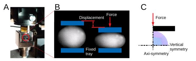
Fig. 1. Global compression test on micropellets. (A) Image of the device used for the mechanical characterization. (B) Schematic representation of the compression test (exaggerated deformation). (C) Symmetry assumptions used with the Finite Element model to estimate the micropellet hyperelastic properties.
